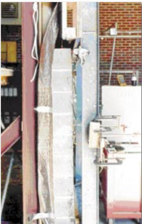
▶ 2 North Carolina A&T State University out-of-plane wall testing – distributed load
